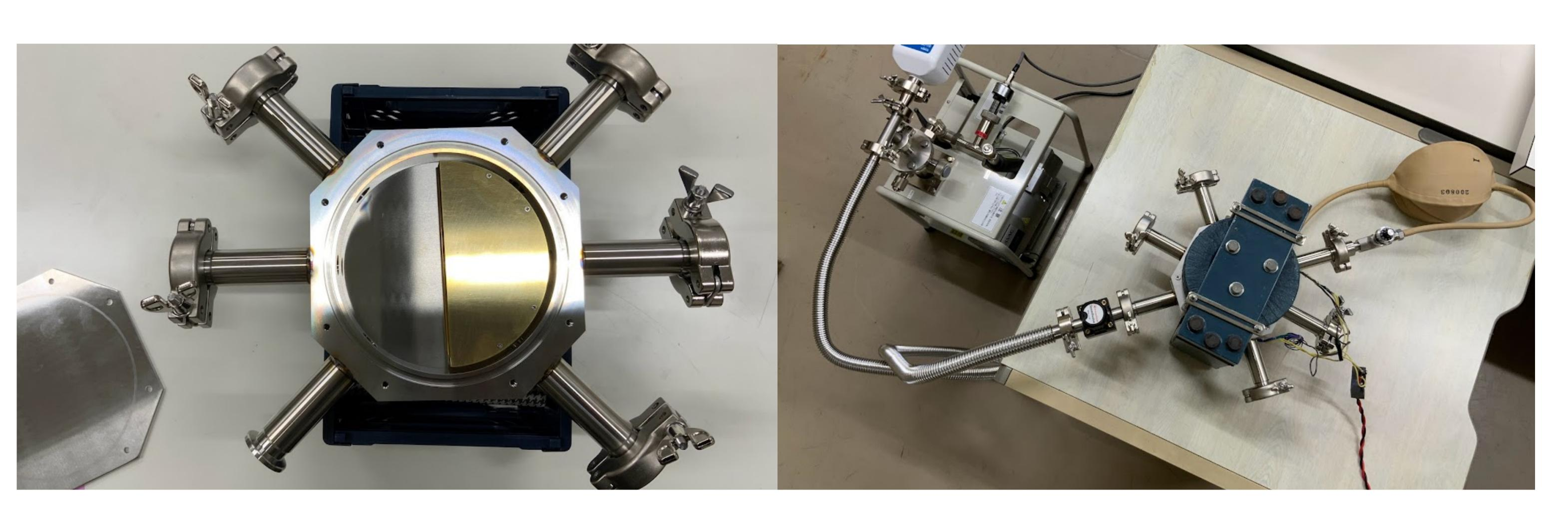
A Dee electrode placed inside the vacuum chamber. Dee electrode is made of a brass and the chamber from stainless steel. Students confirmed that their vacuum reached nearly 9x10<sup>-4</sup> Pa, and it also fits s well in between electromagnets.
