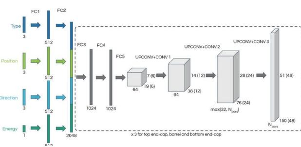
Figure 2. Architecture of the generative neural network used for this work
