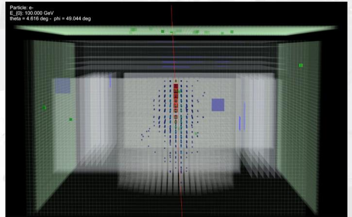
**CALO: 3-d imaging calorimeter:** Energy measurement & Particle identification
