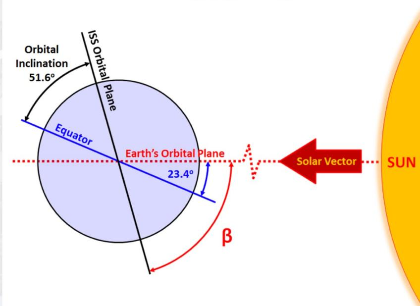
Figure 1. The solar beta angle,  $\beta$ , is the angle between the ISS orbital plane and the solar vector (direction from the Sun to the Earth).
