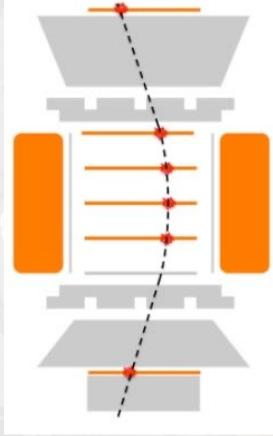
**Inner tracker (layers 2 to 8)** is arranged in a stiff and lightweight carbon shell and cooled by a mechanically pumped CO<sub>2</sub> bi-phase system
