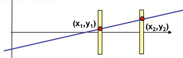
$$\sigma_d^2 = \frac{(r_2\sigma_1)^2 + (r_1\sigma_2)^2}{(r_2 - r_1)^2} + \sigma_{MS}^2$$
