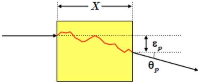
Particles moving through the detector material suffer many e.m. interactions that randomly deviate their trajectory (stochastic process)
