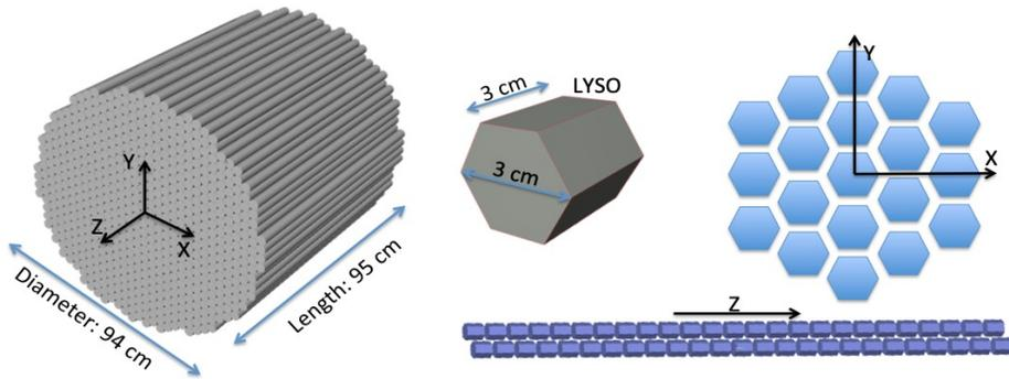
The core: a symmetric LYSO calorimeter with 61  $X_0$  depth
