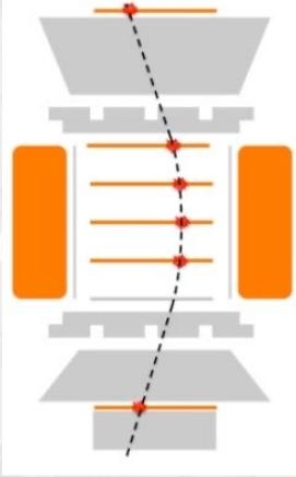
**Inner tracker (layers 2 to 8)** is arranged in a stiff and lightweight carbon shell and cooled by a mechanically pumped CO<sub>2</sub> bi-phase system
