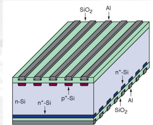
**Scheme of a double-sided microstrip detector (biasing structures not shown):**
