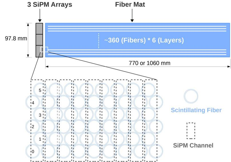
Alternative technology for charge particle tracking based on **SiPM + fiber-bundle coupling**.
