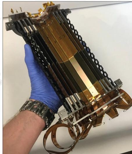
Half of the SLD vertex detector, consisting of 307 Mpixels, three barrels and a pixel size of  $20 \times 20 \times 20 \mu\text{m}^3$ . Each ladder of 16 cm active length contains two 8 cm-long stitched CCDs
