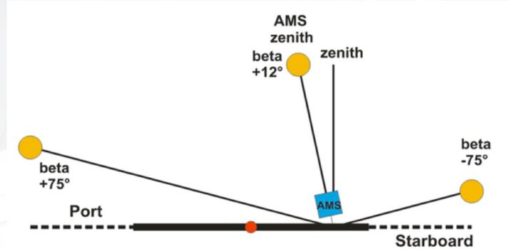
Figure 2. Variation of direction of solar illumination with beta angle. To avoid the rotating ISS solar arrays periodically being in its field of view, AMS is mounted on the ISS with a  $+12^\circ$  "roll" to port.
