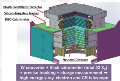
W converter + thick calorimeter (total 33 X<sub>0</sub>)
