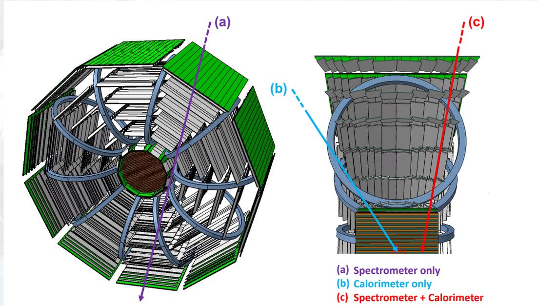
**High Temperature Superconducting (HTS) magnetic spectrometer (SMS)** to measure the particle rigidity, charge magnitude and sign with  $MDR > 20 \text{ TV}$  and acceptance  $> 10 \text{ m}^2 \text{ sr}$
