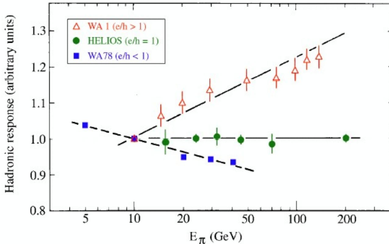
FIG. 3.14. The response to pions as a function of energy for three calorimeters with different  $e/h$  values: the WA1 calorimeter ( $e/h > 1$ , [Abr 81]), the HELIOS calorimeter ( $e/h \approx 1$ , [Ake 87]) and the WA78 calorimeter ( $e/h < 1$ , [Dev 86, Cat 87]). All data are normalized to the results for 10 GeV.
