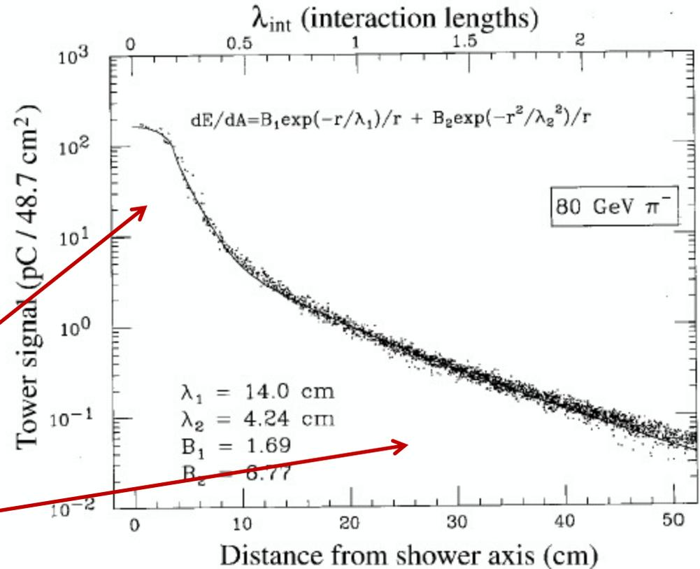
FIG. 2.32. Average lateral profile of the energy deposited by 80 GeV  $\pi^-$  showering in the SPACAL detector. The collected light per unit volume is plotted as a function of the radial distance to the impact point. Data from [Aco 92b].
