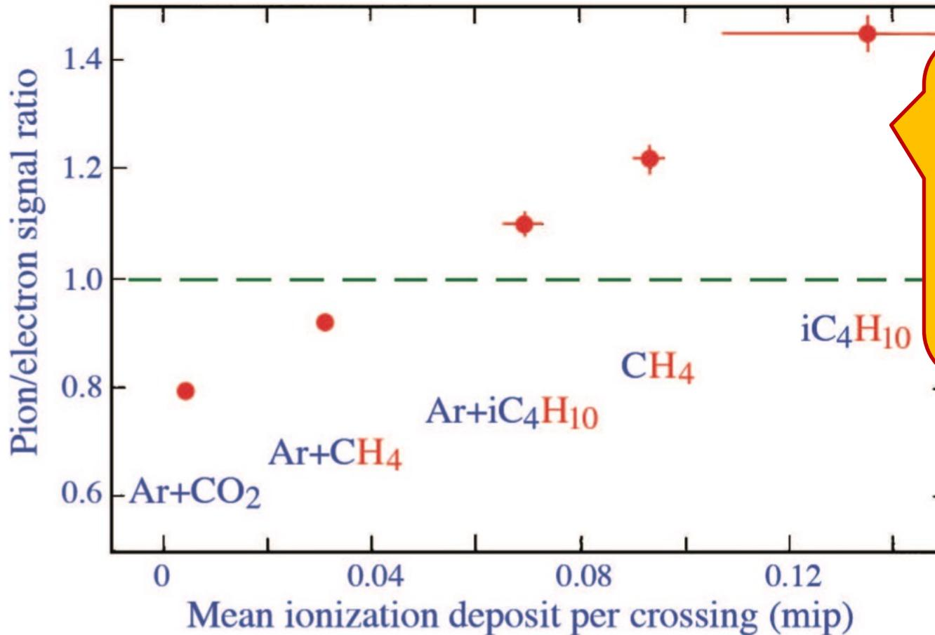
Pion/electron response ratio in the L3 uranium/gas calorimeter as a function of the hydrogen content of the gas mixture.
