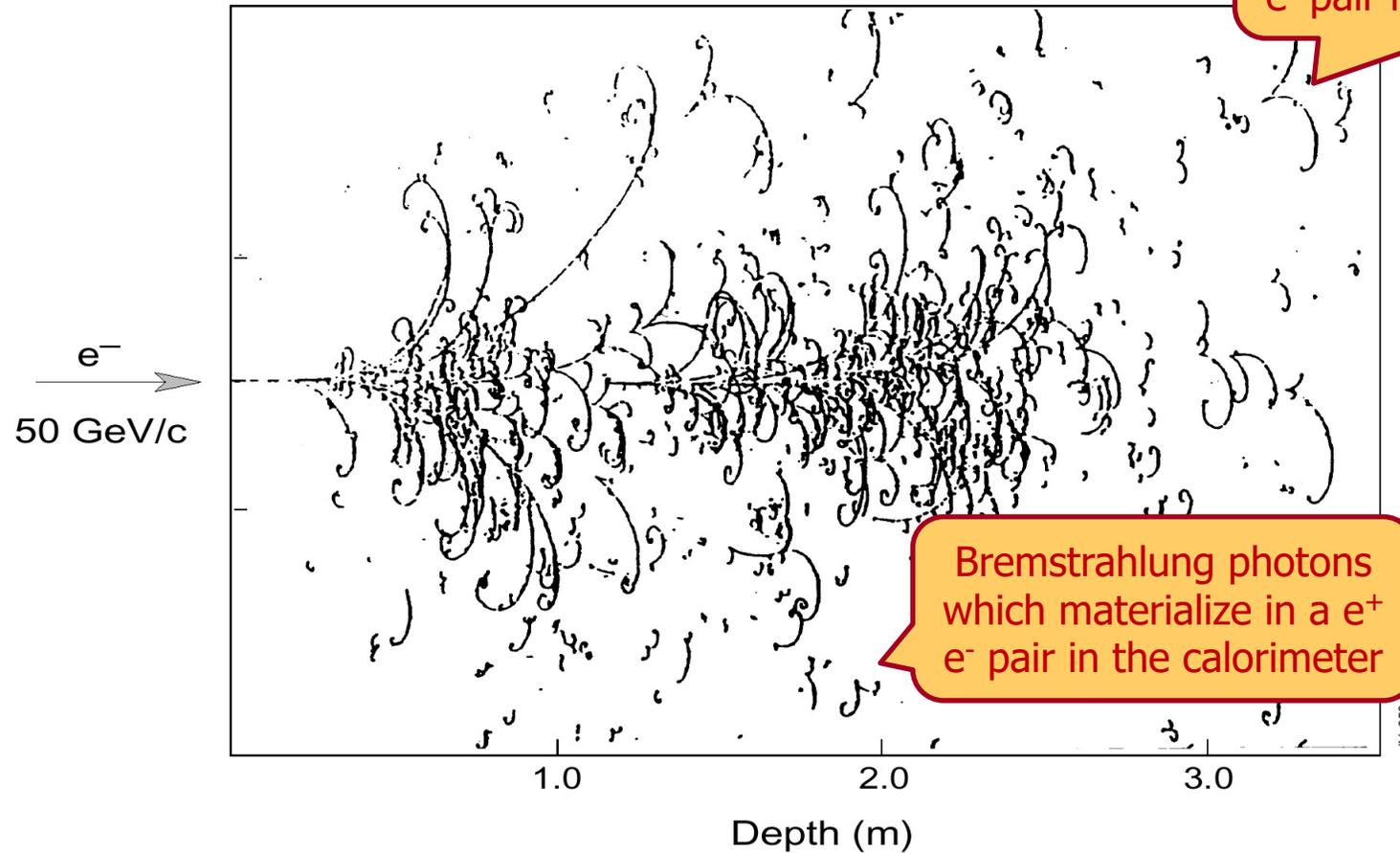
Big European Bubble Chamber filled with Ne:H<sub>2</sub> (70%:30%), 3T field, L=3.5m,  $X_0=34 \text{ cm}$ , 50 GeV incident electron
