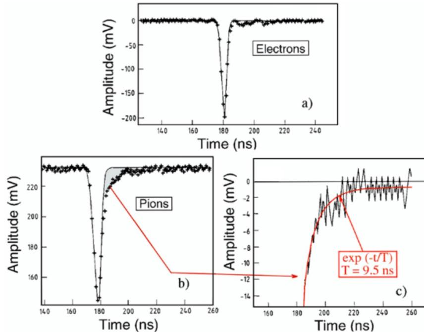
FIG. 3.22. Typical calorimeter signals for 150 GeV electrons (a) and pions (b) measured with the SPACAL calorimeter. The pion signal exhibits a clear exponential tail with a time constant of  $\sim 10$  ns (c). The  $t = 0$  point is arbitrary and the bin size is 1 ns. Data from [Aco 91a].
