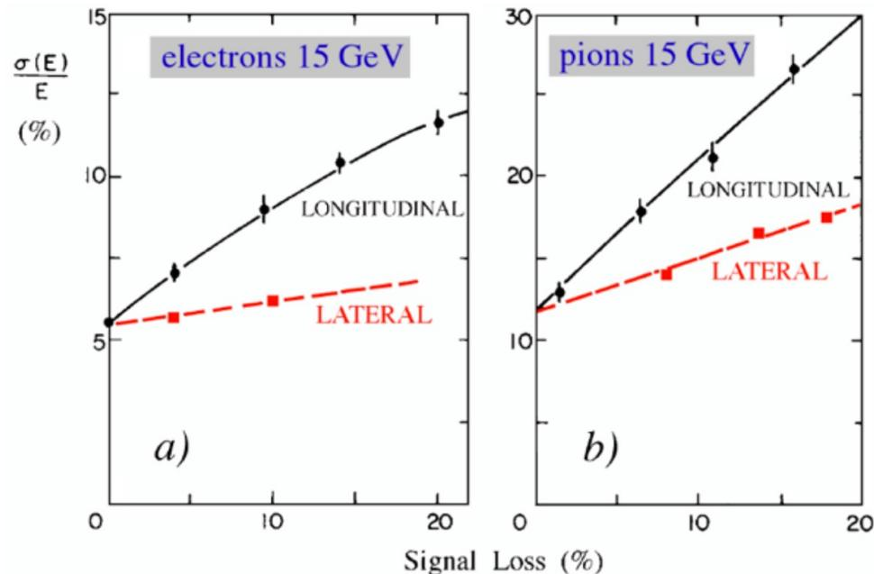
FIG. 4.33. The effects of longitudinal and lateral shower leakage on the energy resolution, as measured for 15 GeV electrons (a) and pions (b) by the CHARM Collaboration in a low- $Z$  calorimeter [Did 80, Amal 81].
