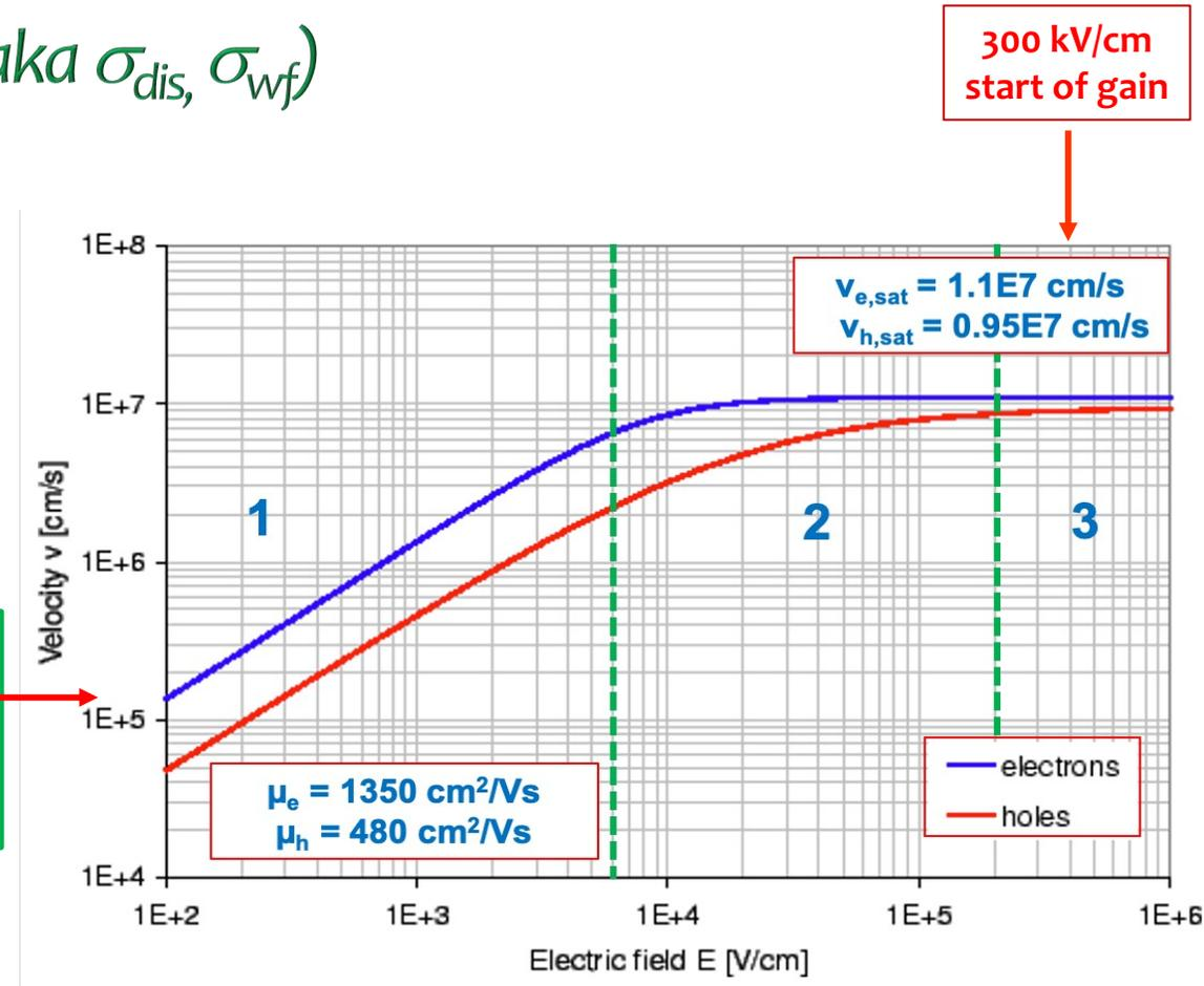
Carrier velocities vs electric field in silicon:
