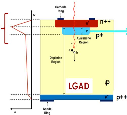
Thin, highly doped, p-implant near the p-n junction
