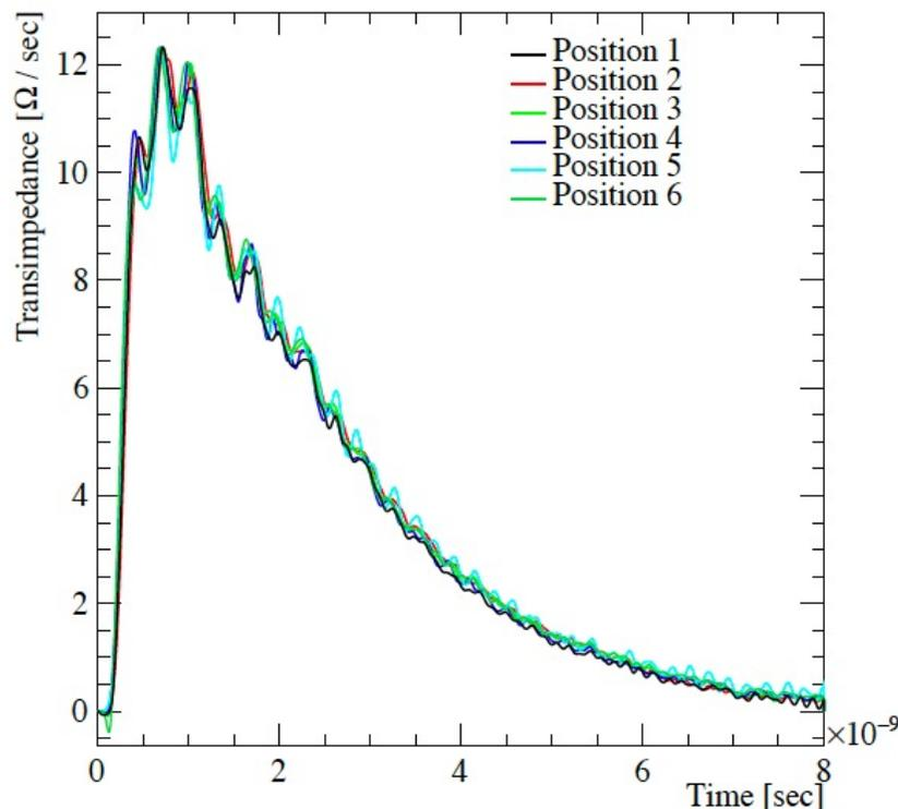
Comparison of semiempirical transfer functions obtained in different irradiation positions with the laser setup, for the -150V bias sample.
