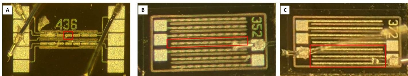
Tested structures. For each sensor the active area is shown in red. (A) Single pixels sensor; (B) strip sensor; (C) triple strip sensor
