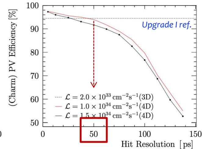
**50 ps per hit (corresponding to 20 ps per track) are sufficient to recover the Upgrade-I efficiency**
