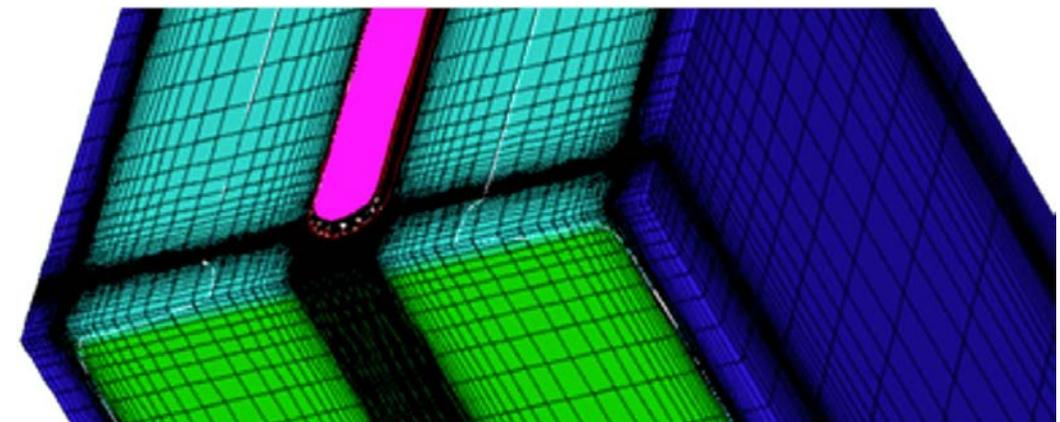
3D-silicon sensor with highlighted tensorial mesh grid.
