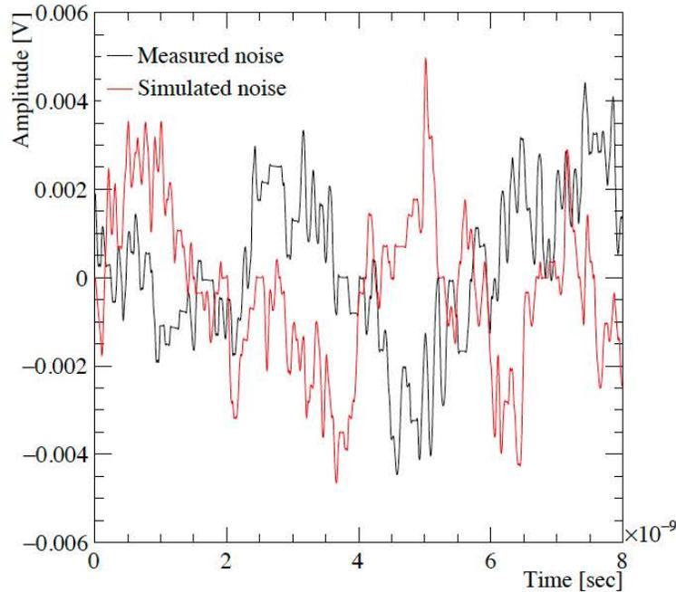
Comparison between two waveforms of (black) measured and (red) simulated noise for the -150V bias sample
