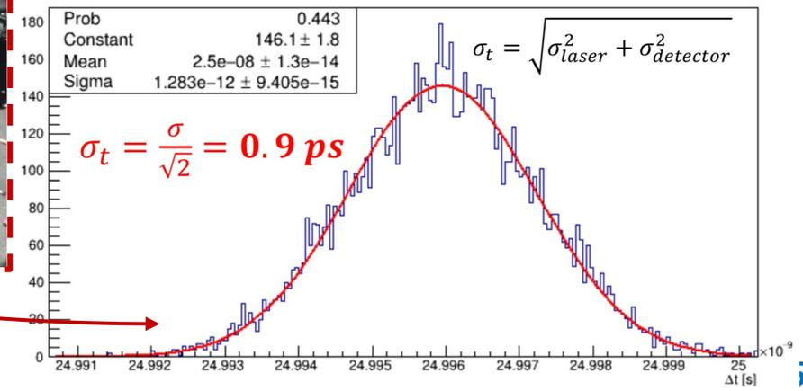
By choosing the waist shape (changing optics) and properly calibrating the laser intensity (using a precision CSA) a MIP-like deposit is generated
