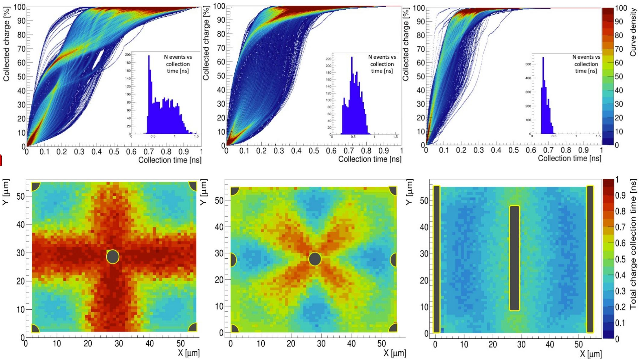
Time performance comparison among three different 3D geometries at  $V_{bias} = -100V$  (from left to right: five columns, nine columns and trench geometry). (Top) percentage of total charge collected on the electrodes versus time. (Top inserts) distribution of charge collection time for the three geometries. (Bottom) time for complete charge collection versus impact point for the same geometries. Each simulation is based on about 3 000 MIP tracks.
