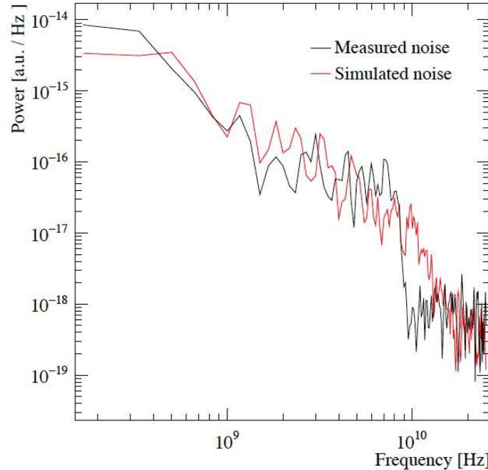
Noise waveform in time domain: power spectral densities
