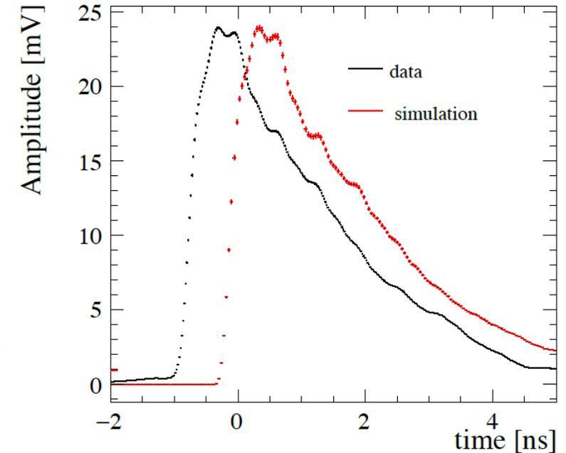
Silicon sensor average waveform from the full (black) data and (red) simulation sample (about 30000 signals). An arbitrary time shift between the two shapes is applied to allow a qualitative comparison
