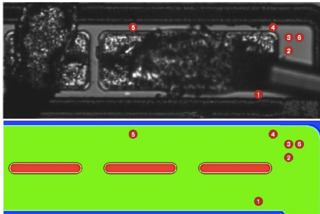
Six irradiation positions within the active area of the actual double-pixel test structure (top) and the corresponding positions in the simulated structure (bottom).
