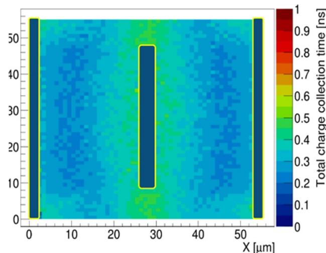
Simulated Time of arrival map of a single 3D-trench sensor pixel obtained in the lab by IR laser scan ( $\alpha_{\text{tilt}} = 0^\circ$ )
