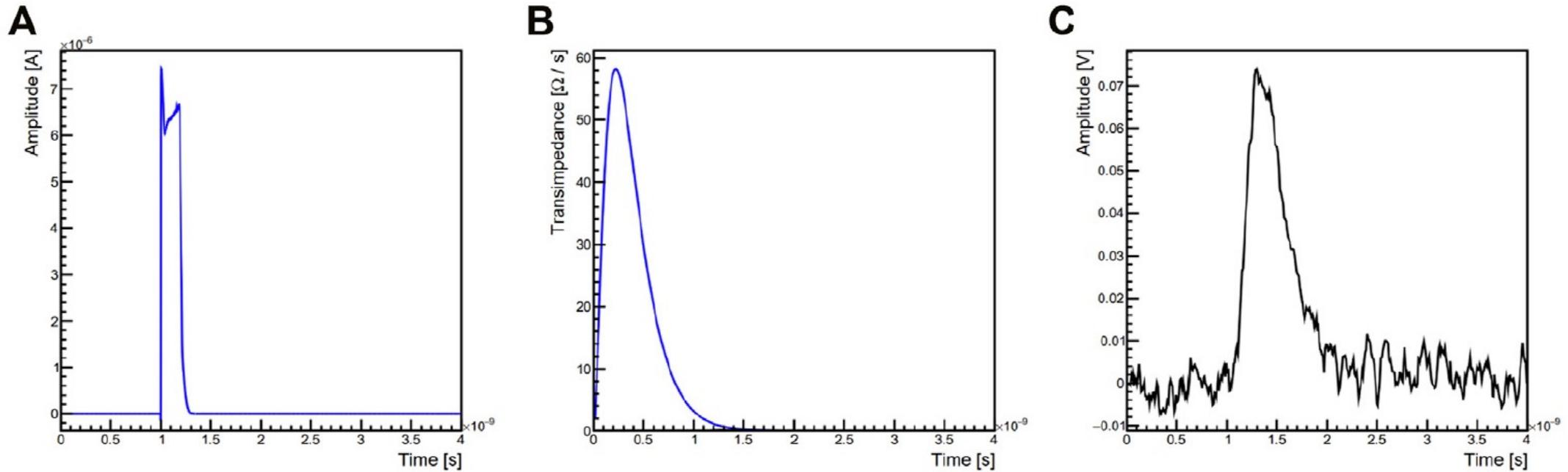
Example of the result of the front-end simulation for a single input current from TCoDe, for a 3D-trench double pixel structure at -150 V bias voltage:
