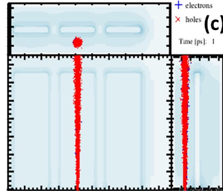
Examples of calculated energy deposit shapes **from laser sources** inside a TimeSPOT 3D-trench structure:
