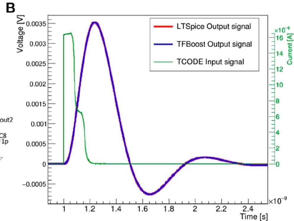
Spice simulation of a circuit that uses the spice model of a real SiGe bipolar transistor
