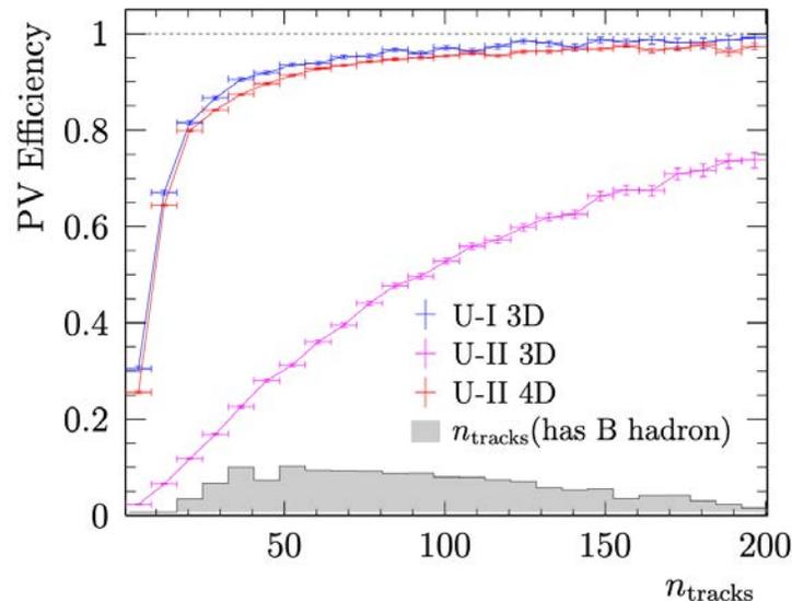
**Reconstruction efficiency vs the number of tracks per primary vertex, comparing the Upgrade I 3D reconstruction in both data conditions, and a variant using timing information to resolve the primary vertices**
