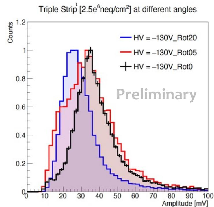
The inefficiency (at normal incidence) due to the dead-area of the trenches is fully recovered by tilting the sensors around the trench axis
