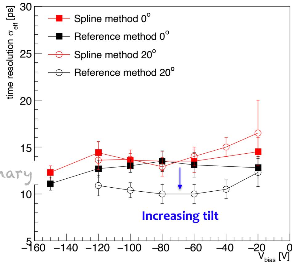
Excellent time resolution ( $\sigma_{\text{eff}} = 11 \text{ ps}$ ) measured at 150V on single pixels irradiated with fluences of  $2.5 \cdot 10^{16} \text{ 1-MeV } n_{\text{eq}}/\text{cm}^2$
