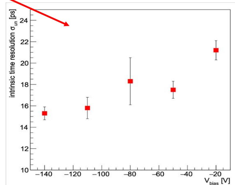
Intrinsic time resolution of a 3D-trench sensor  $\sigma_{un}$  (right) and contribution of the electronic jitter  $\sigma_{ej}$  (left) vs bias Voltage.
