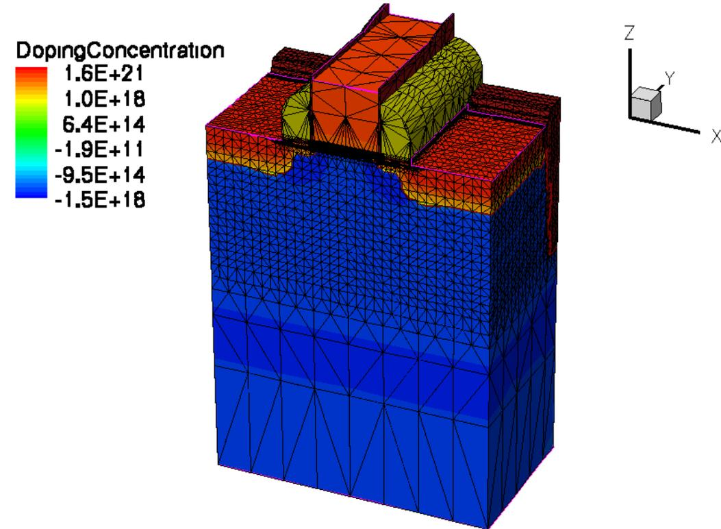
A CMOS transistor in TCAD, with highlighted tensorial mesh grid.
