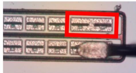
double pixel  $55 \times 110 \mu\text{m}^2$
