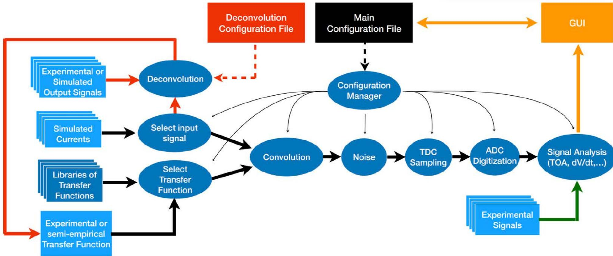
**TFBoost simulations flow.** The black path is the main simulation in which the convolution and the signal analysis are performed. The green path is followed if TFBoost is used as a pure signal analyzer, while the red path is followed to perform the deconvolution between an input current and an output signal.
