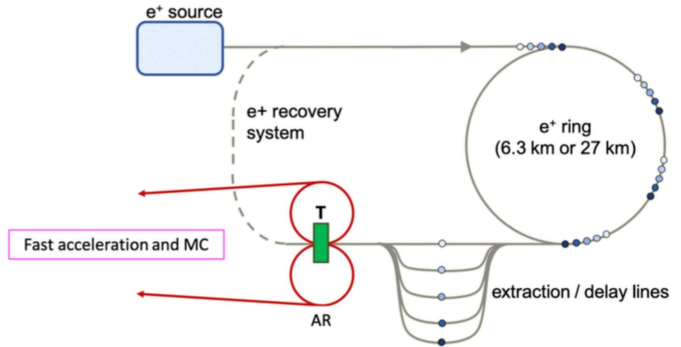
Target insertion embedded in the positron ring
