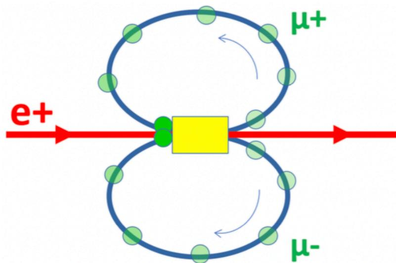
A dedicated muon **production** and **accumulation system** is one of the most important features of the LEMMA design.
