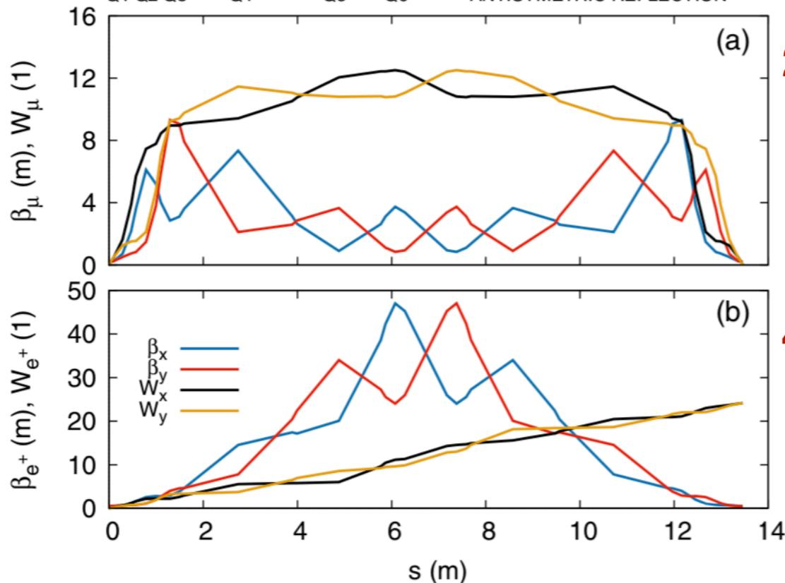
The line must be able to **transport 3 beams** ( $e^+$ ,  $\mu^+$ ,  $\mu^-$ )
