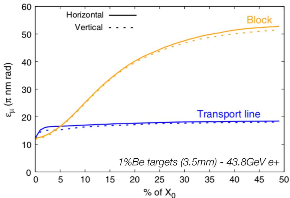
The line proves **very effective** in transporting the muon beam through several targets while keeping the **emittance constant**.
