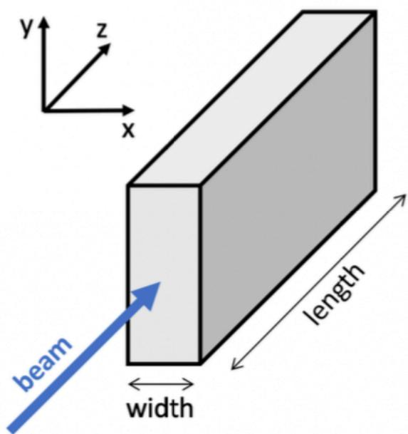
Target features are width, length and material.
