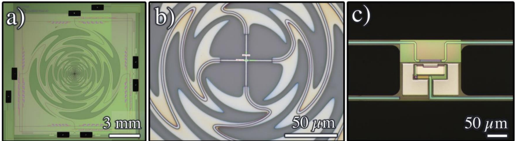
Fig. 3 a LF-1 prototype pixel with sinuous antenna in the center, the microstrip transmission line is routed between antenna arms, bandpass filters with mitered stubs surround the antenna, and the bolometers appear as rectangles. b Antenna feedline coupling with line widths at the center of 600 \pm 50 nm. c The bolometer island with TES in the center, thermal ballast on the lower half of the island, readout wires routed to the lower right split the ballast, and antenna feedlines in the upper left and right lead to the load resistor above the TES (Color figure online)
