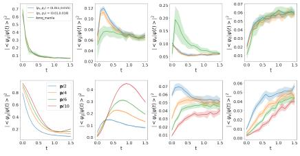
ibmq\_manila: dephasing time  $T_2 \approx 60 \ \mu s$ , gate time  $\approx 370 \pm 80 \ ns$ max circuit moments  $= \frac{T_2}{\text{gate time}} \approx 160$ Trotter step with 20 moments  $\Rightarrow$  ground state preparation
