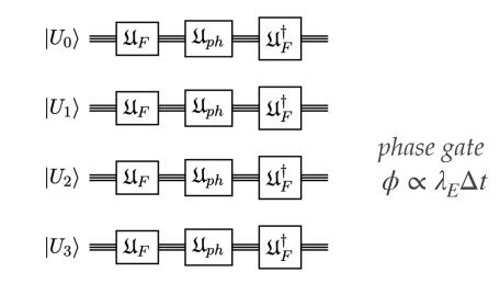
Circuit realizing the time evolution of 4 links generated by  $H_E$ .
