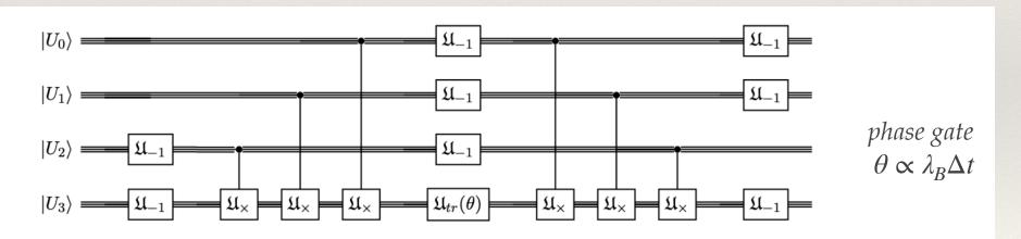
Quantum circuit realizing the time evolution of a single plaquette generated by the magnetic term of the hamiltonian. In summary, the steps of the calculations are:
