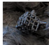
Sintered component at 1450°C
