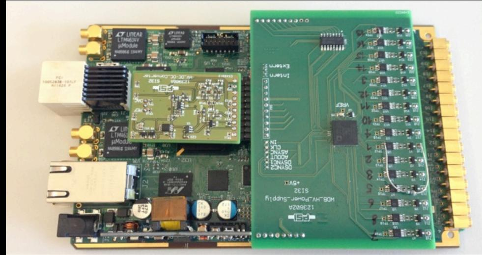
16 channels data acquisition board designed and used by the MEG2 experiment at PSI ( $\mu \rightarrow e + \gamma$ )
