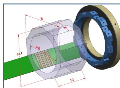
We already built this PET insert based on a single monolithic scintillator LYSO tube with inner circular face but ten outer facets (2).
