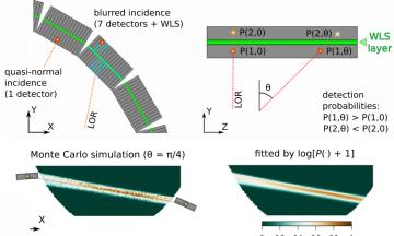
Shift-variant SRM  $\chi_{i_{\epsilon}}(x_j, y_j, z_j, \Delta t_{\epsilon}, \theta)$ : 2D Monte Carlo – emissions on transverse planes for various obliqueness  $\theta \rightarrow$  express SRM as log-polynomial fitting functions, + kernels for TOF, parallax correction and Z.
