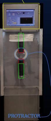
The two scintillators detect cosmic rays coming into the apparatus.
