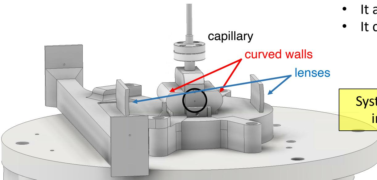
System to compensate for laser phase shift induced by circular channel geometry
