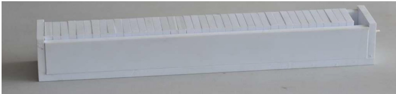
Blocks of polystyrene (10 mm) + Fuji film detectors (40x40 mm 2 )
