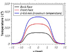
With a parabolic heat distribution we decrease the density power on the inner disk regions, which are the most difficult to be cooled due to the low thermal conductivity. In case of a single cooled face, however, it is convenient to adopt an exponential-like distribution.
