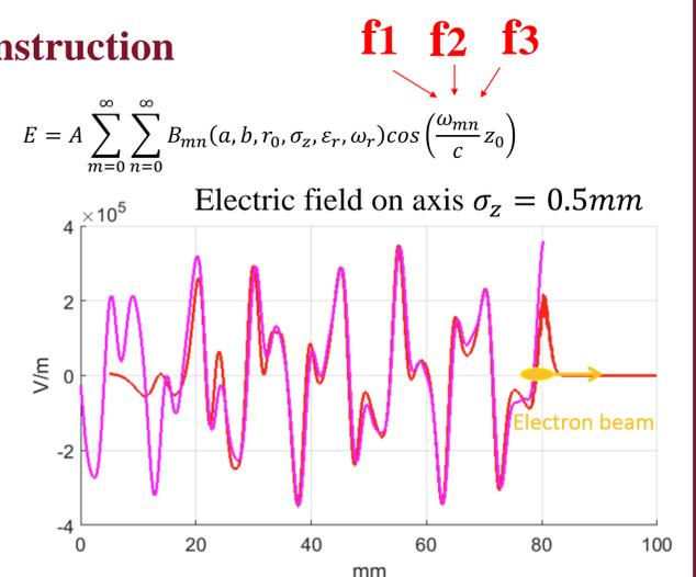
$E_z$  behind the electron beam with a  $\sigma_z = 1 \text{ mm}$ . PIC results (red), sum of the first three TM<sub>0n</sub> modes (magenta)
