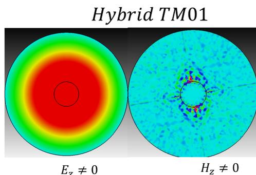
A generic hybrid TM mode could have a longitudinal component of the magnetic field
