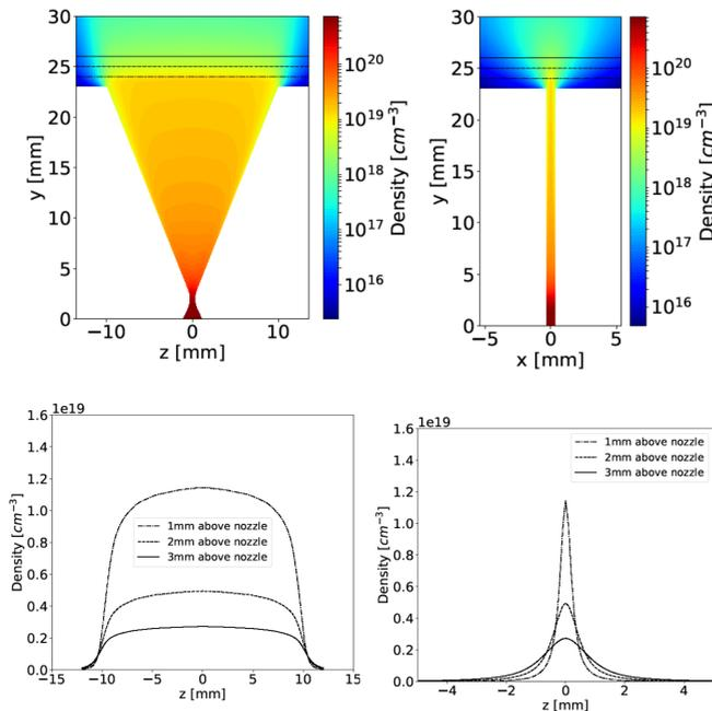
Density profiles along laser propagation direction (left) and in transverse direction (right) in different heights over the nozzle
