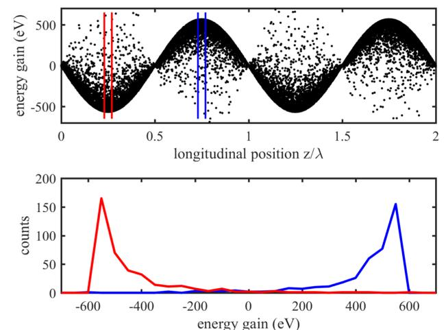
Figure: Laser-induced energy modulation in a dipole magnet. Top: energy versus position  $z/\lambda$ . Bottom: Marked distributions.
