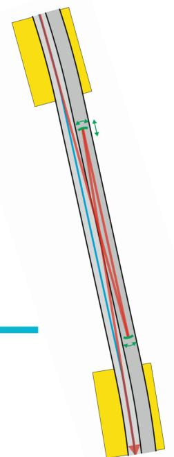
Figure: Laser guided from one dipole to the next by 2 mirrors controlling position, angle and laser phase (see arrows).
