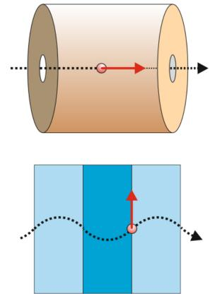
Figure: RF cavity (top) with longitudinal electric field and undulator (bottom) with transverse electric laser field
