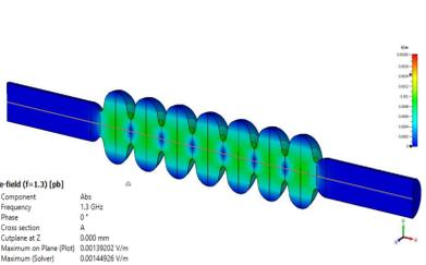
Field profile in the 7-cell cavity simulated by SUPERFISH
