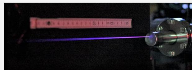
Fluorescence of 2.7 keV photon beam at XFEL
