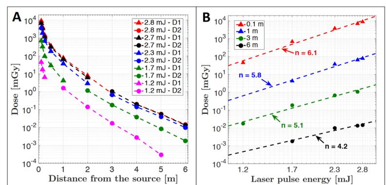
Measured radiation doses for 1 minute at 100 Hz with laser focus in air. Image from [2]
