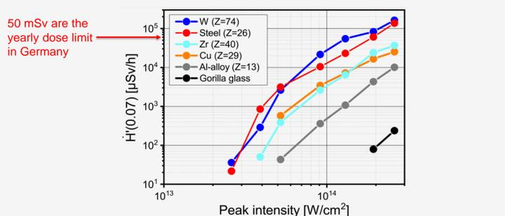
Dose rate from 40 W laser for different Materials (10µm, 100µJ, 400kHz). Image from [1]
