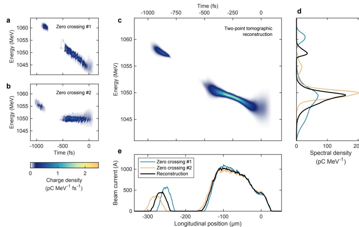
Longitudinal phase space measured with PolariX transverse deflection structure (TDS).
