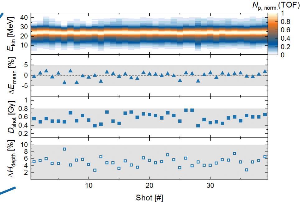
Enabling a full-scale pilot study in a small animal model with a laser proton beam
