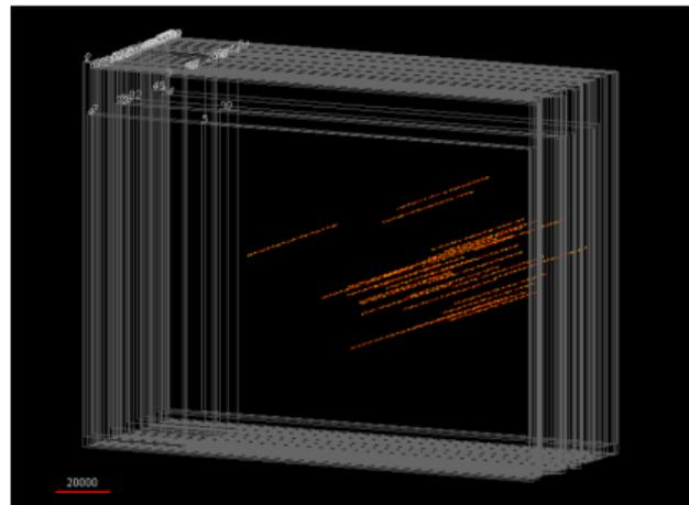
*Simulated muons reconstructed in the emulsion target*
