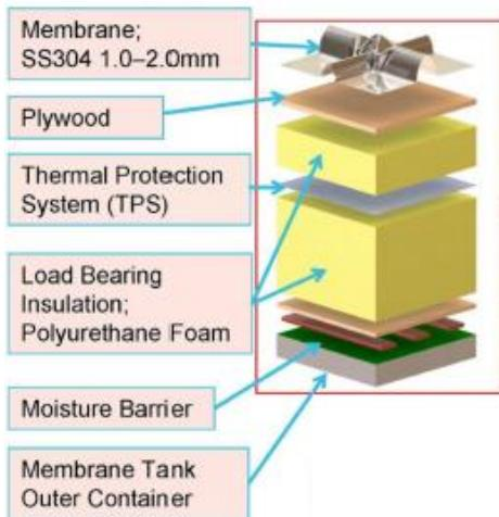
Construction of the cryostat will
