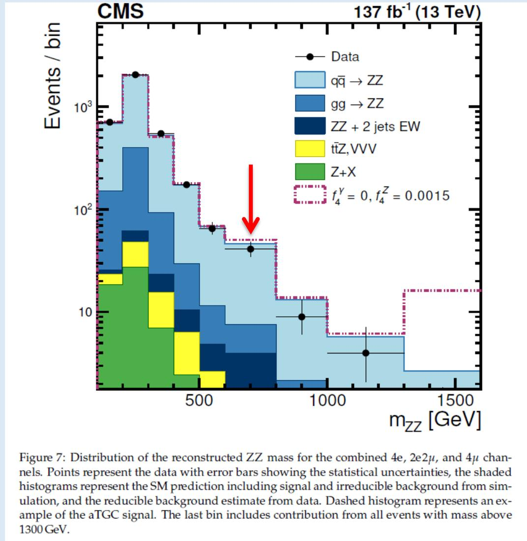
Figure 7: Distribution of the reconstructed ZZ mass for the combined 4e, 2e2 $\mu$ , and 4 $\mu$  channels. Points represent the data with error bars showing the statistical uncertainties, the shaded histograms represent the SM prediction including signal and irreducible background from simulation, and the reducible background estimate from data. Dashed histogram represents an example of the aTGC signal. The last bin includes contribution from all events with mass above 1300 GeV.
