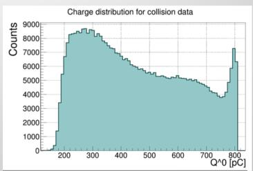
The SiPM voltage has been set as high as possible to clearly observe the MIP values. A saturation of the charge spectrum for collision data has been observed.
