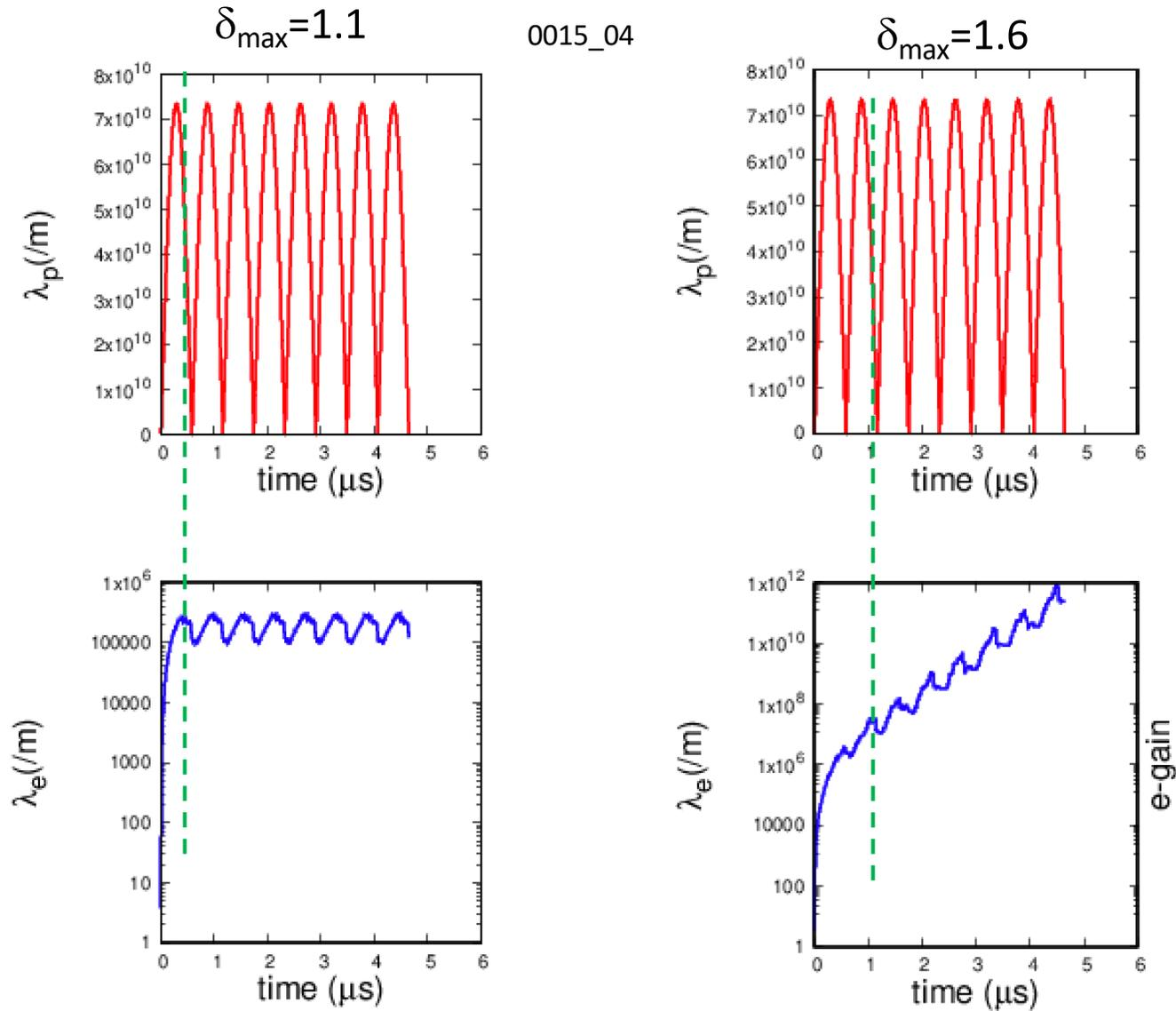
Electron generation peak is delayed from proton peak (trailing edge multipacting)
