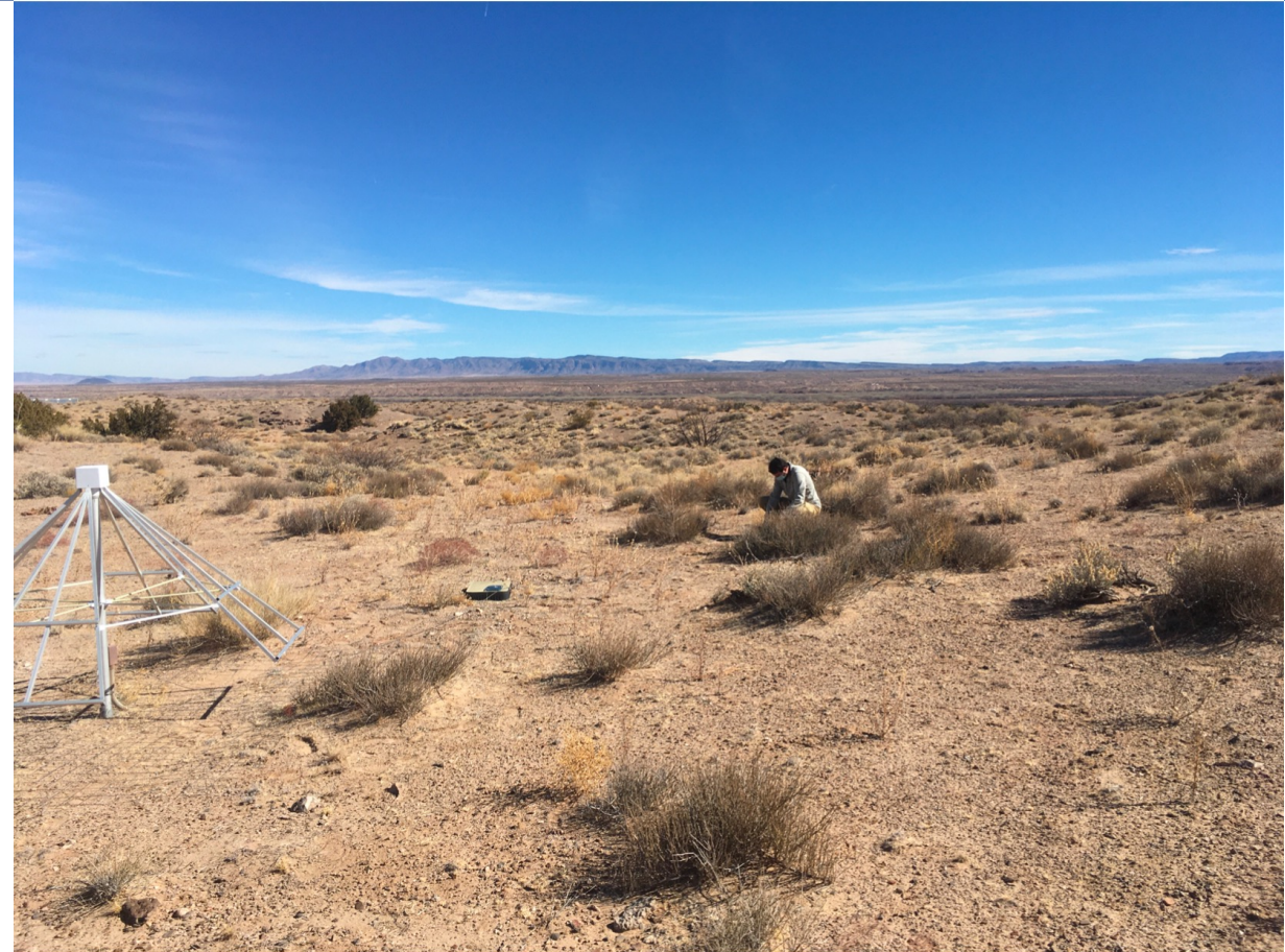
In situ measurements of the LWA antenna impedance using a VNA
