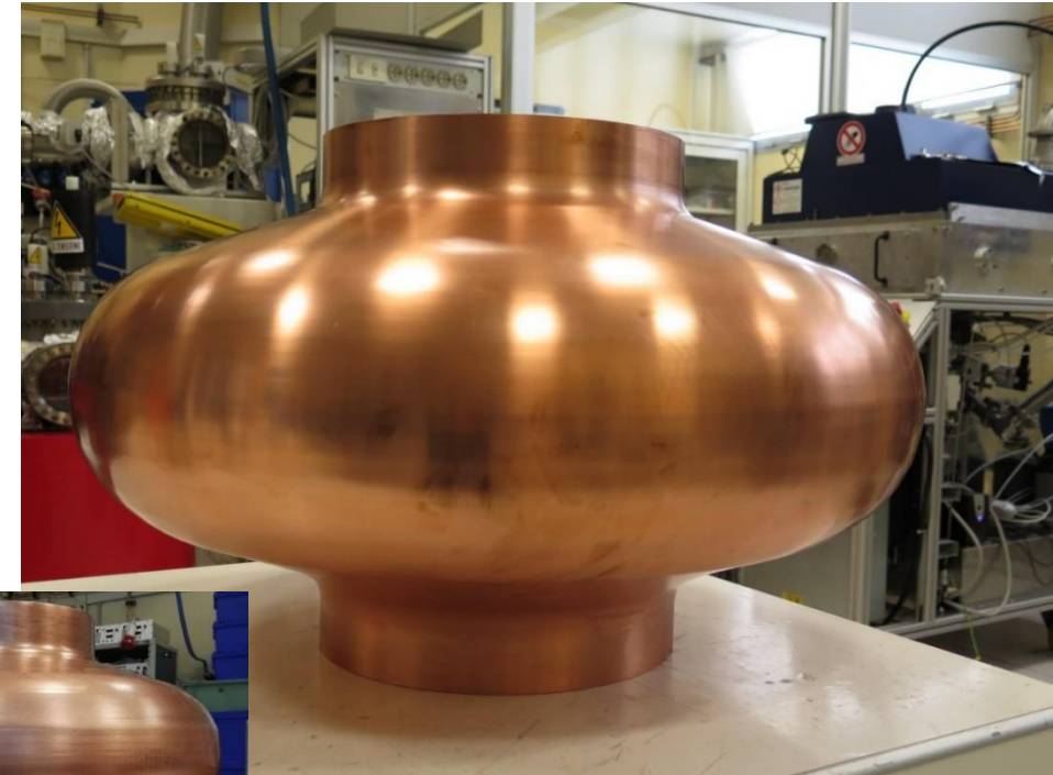
Spinning of Cavity #2 completed
