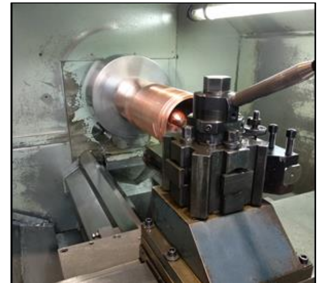
QWR cavity machining
