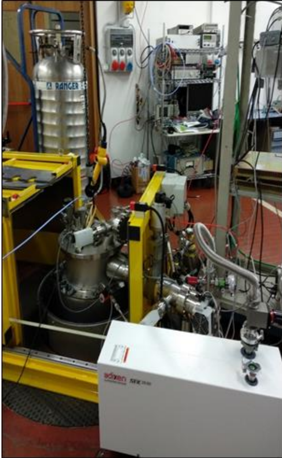
Cryostat for offline measurement test
