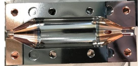
NbTi haloscope developed in QUAX at LNL/LNF
