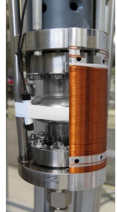
Trapped Flux measurements on 6 GHz cavities
