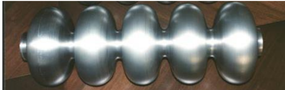
First seamless multicell by spinning
