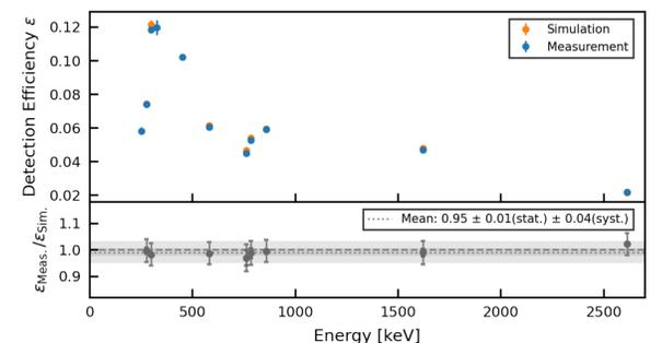
Verification of the detection efficiency simulations with a calibrated Th-228 point source.
