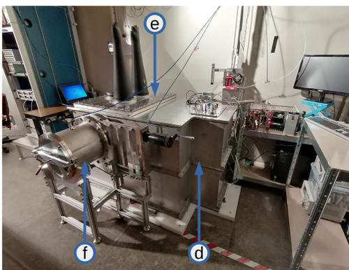
(a) HPGe crystal inside Cu cryostat, (b) OFHC Cu cavity, (c) lead shield, (d) airtight enclosure, (e) glove ports, (f) sample load lock
