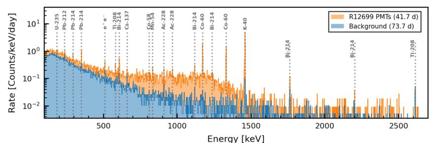
Measured energy spectrum of sample photosensors (orange) as compared to the background (blue). Prominent isotopes are labeled.
