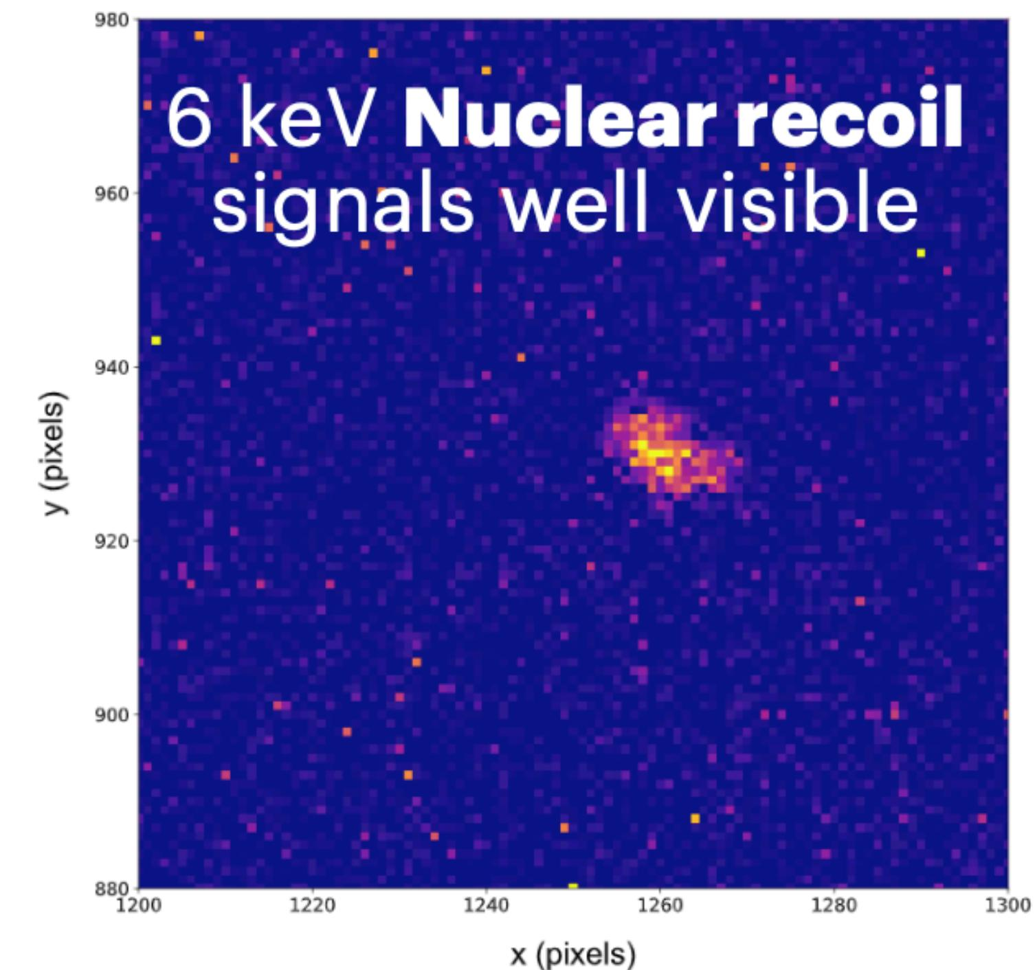
40% nuclear recoil efficiency at 6 keV<sub>ee</sub> with 96% rejection against  ${}^{55}\text{Fe}$
