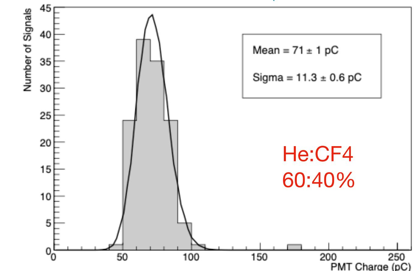
Energy resolution of 15% at 5.9 keV<sub>ee</sub> with sCMOS and PMT
