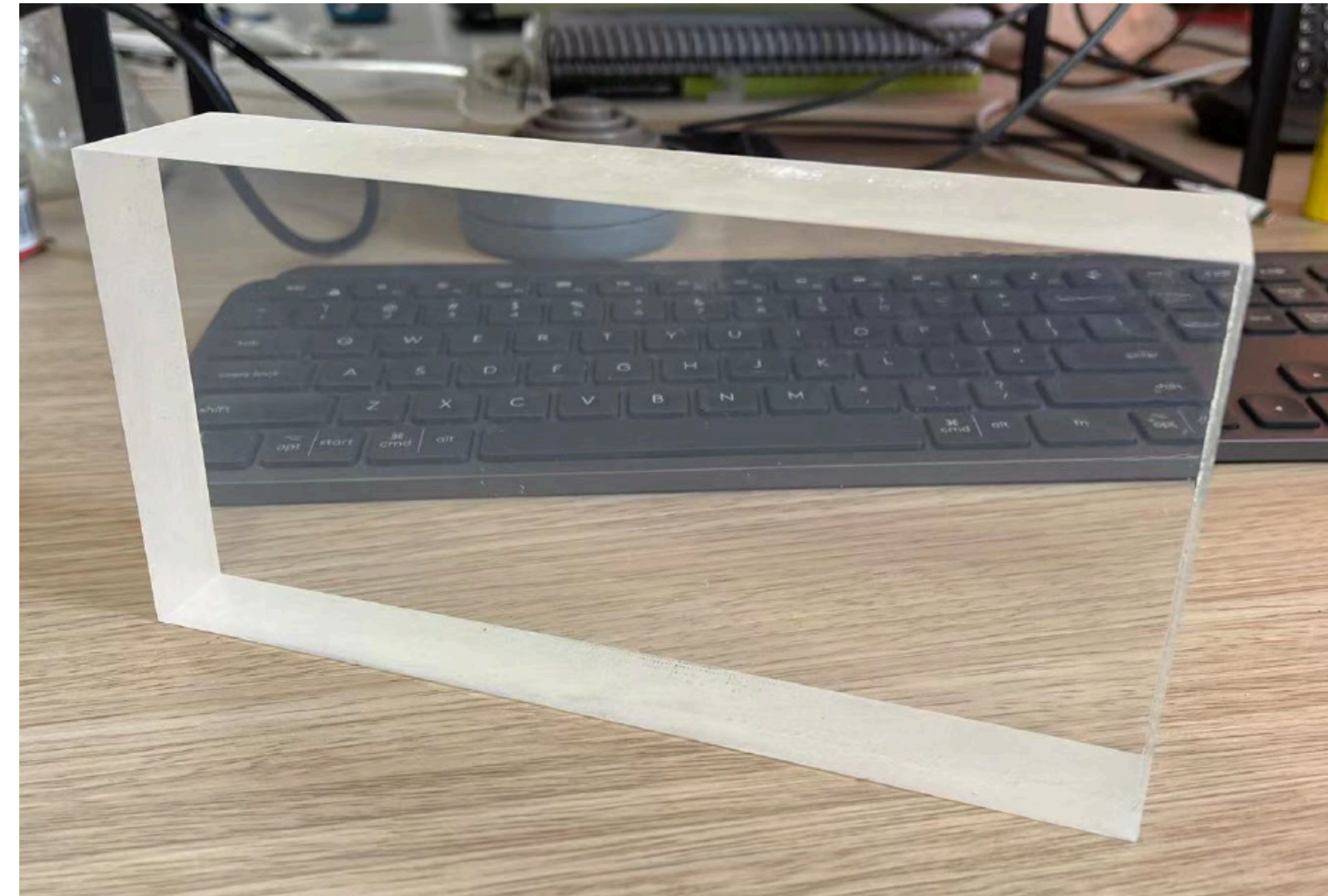
\text{Gd(MAA)}_3 doped acrylic sheet (5 cm thick)
