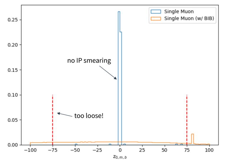
Will tighten to ±1 mm around IP.
