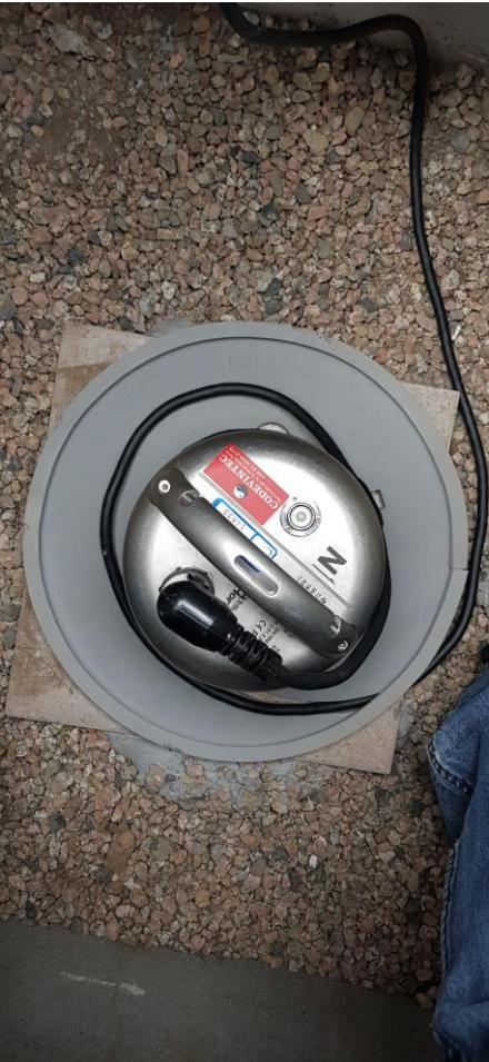
As surface reference we deployed two **Trillium 120 Horizon** in a vault installation. In both cases, the digitizers are running with an input range of 4Vpp.
