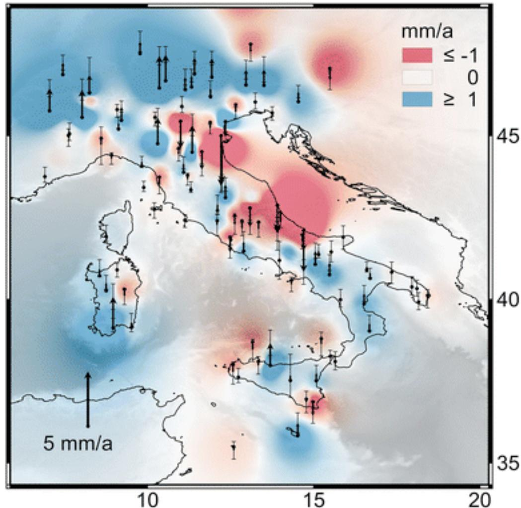
Vertical velocities and error bars with 95 % confidence level. The interpolated vertical velocity field is displayed by a graduated color scale. White represents stable area, blue is for uplift  $\geq 1.0$  mm/a and red subsidence  $\leq -1.0$  mm/a
