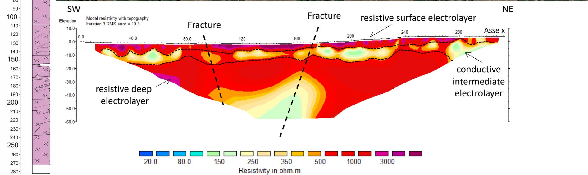
The tomography of the Bitti vertex shows a stratified resistivity array composed of:
