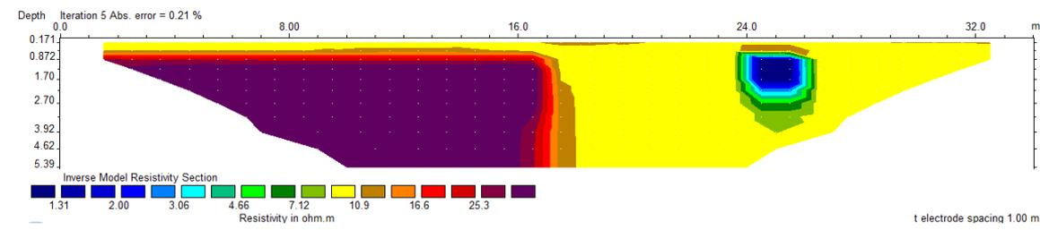
**Tomography** = high resolution subsurface geological model with **calculated** resistivity values.
