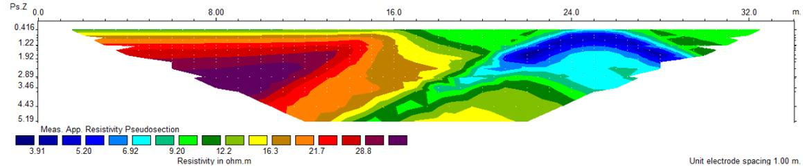
**Pseudosection** = Approximate picture of the true subsurface resistivity distribution beneath the survey line with **measured** resistivity values.
