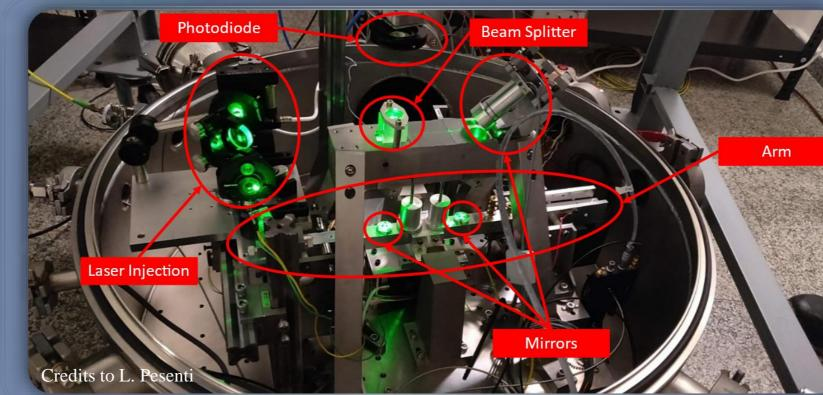
The Archimedes' Prototype **mechanics** consists in a 50 cm long arm with low momentum of inertia suspended through thin flexible joints (100  $\mu$ m x 500  $\mu$ m). Depending on the center of mass positioning, its resonance frequency is around 20-30 mHz. At the ends of the arm, there are two actuators needed to keep the arm in balance.
