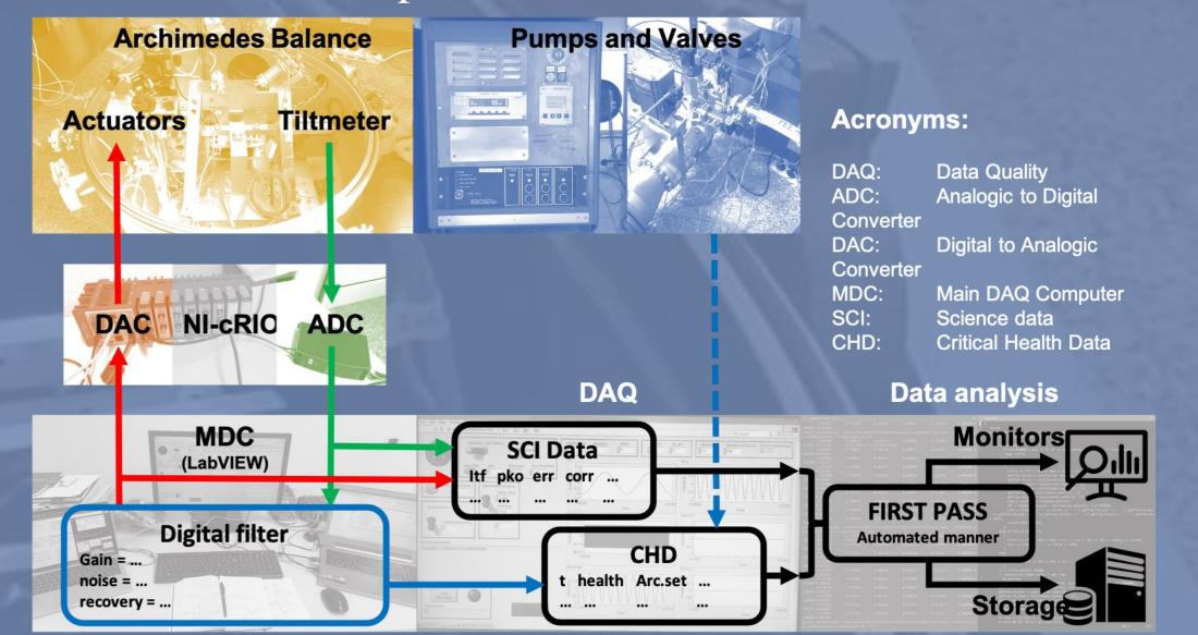
The Archimedes' prototype was used as a **tiltmeter** at Virgo while reached the sensitivity of the sub-picoradiant in the frequency region between 2 and 20 Hz at Sos-Enattos.
