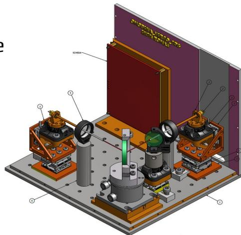
*HD detector measures the level of produced squeezing w.r.t a bright local oscillator (LO)*
