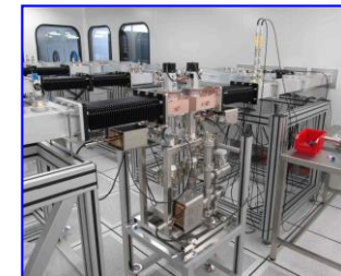
Clean rooms RF couplers and conditioning bench
