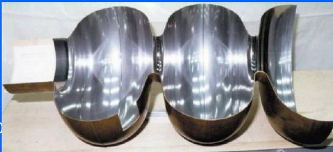
Cut of a 352 MHz niobium coated SC cavity
