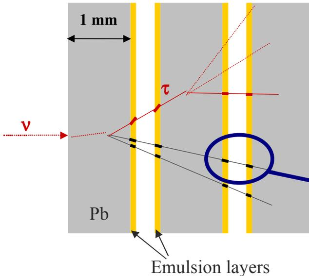
1 mm thick Pb layers interleaved with emulsions
