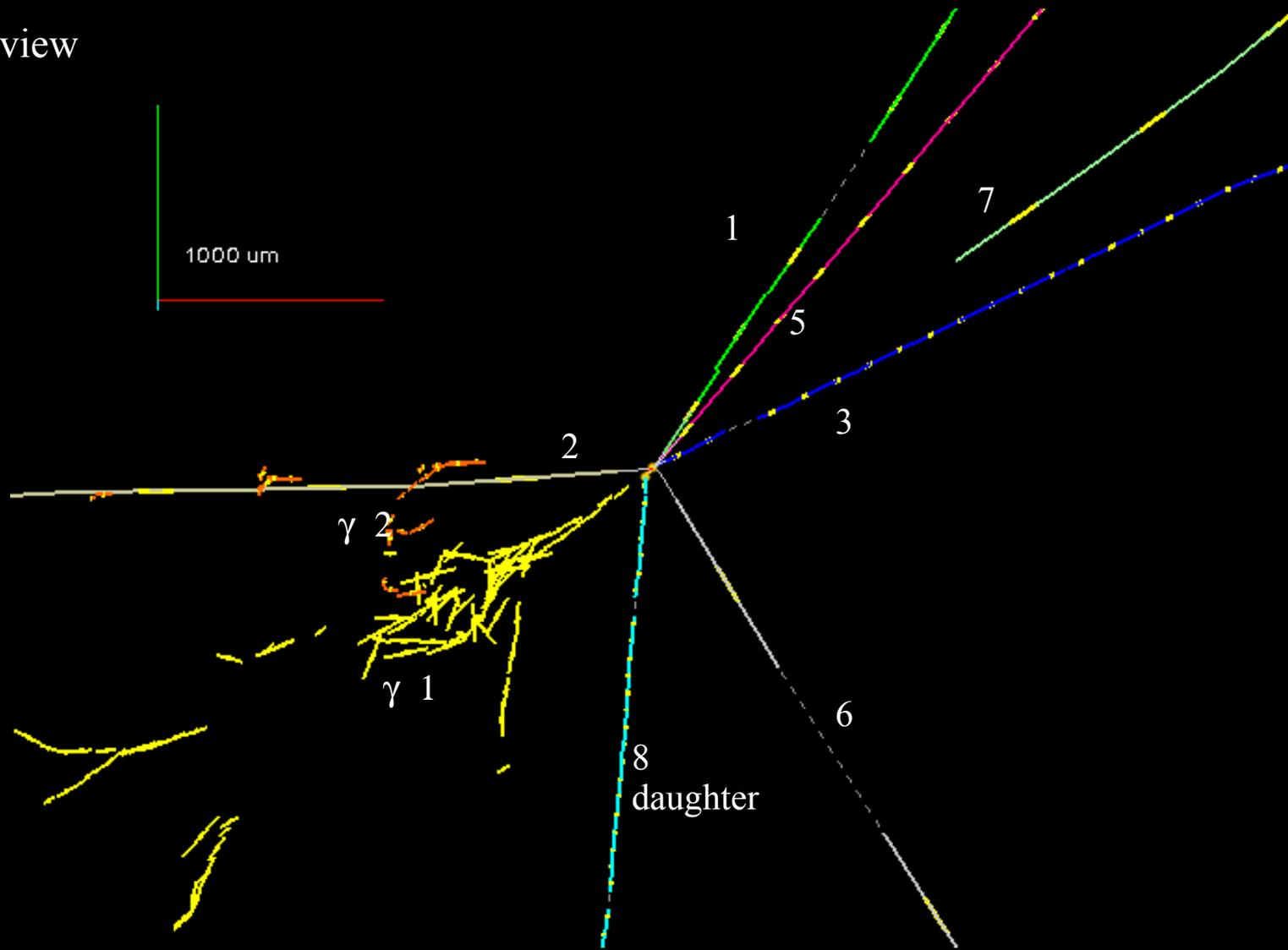
Vertex tracks followed down (through several bricks) to assess the muonless nature of the event. Residual probability of  $\nu_{\mu}$  CC event (due to a possibly undetected large angle muon)  $\sim 1\%$ . **“Nominal” value of 5% assumed**
