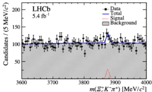
Figure 2: Invariant mass  $m(\Xi_c^+ K^- \pi^+)$  distribution of selected  $\Omega_{cc}^+$  candidates from (black points) selection A, with (blue solid line) the fit with the largest local significance at the mass of 3876 MeV/c<sup>2</sup> superimposed.
