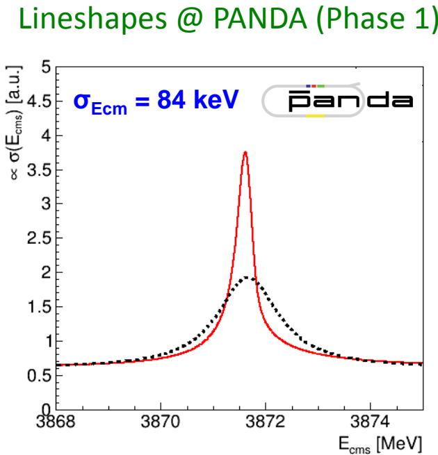
Due to precise beam resolution  $O(50 - 100 \text{ keV})$  @ PANDA
