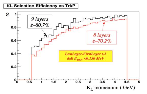
Performed a Very Loose  $K_L$  selector to compare configuration with 8 and 9 active layers  $\rightarrow$  Configuration with 9 layer gives better  $K_L$  efficiency -Need to simulate background samples to have meaningful results, but it's a good start
