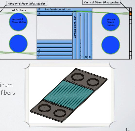
• The boxes are made of aluminum and will contains scintillators, fibers and the photodetectors.
