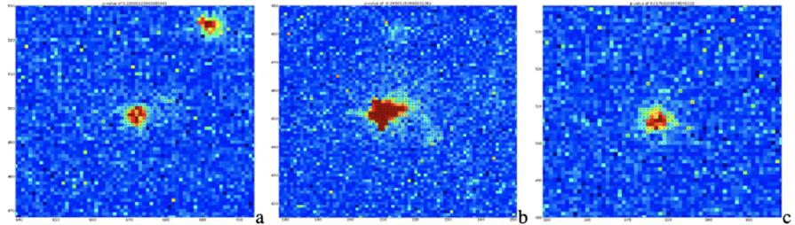
Figure 16: Examples of cluster with a correlation index  $< |0.6|$ . The pixels identified as part of the cluster are indicated with a red dot. (a) p-value of  $0.22$ ; (b) p-value of  $0.24$ ; (c) p-value of  $0.018$ .
