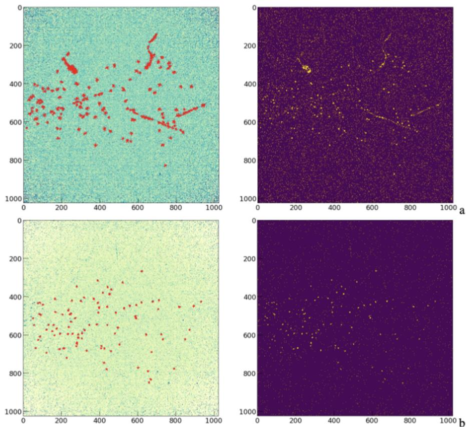
Figure 30: Comparison of two images reconstructed by the DBSCAN algorithm with the same DBSCAN parameters. The image (a) is the image number 90 of the run 4062, while the image (b) is the image number 0 of the run 4069. The right side of the images are the over threshold pixels of the image.
