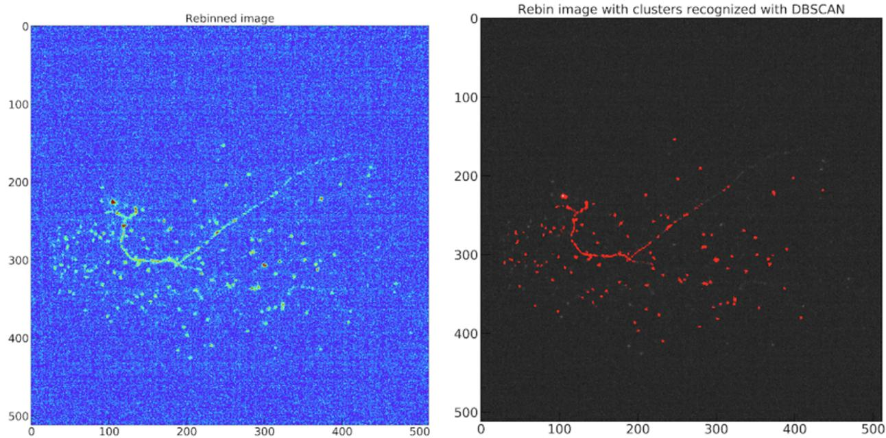
Figure 14: *Example of DBSCAN's cluster recognition on a sample image of He-CF<sub>4</sub> with our choice of parameters. The first image is the raw rebinned image of the signal, while the second one is a black and white version with the position of the recognized cluster superimposed in red.*
