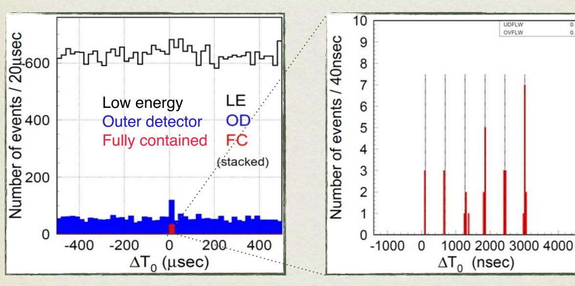
Out-of-time OD/LE rate is flat. No out-of-time FC events. GPS system is working correctly
