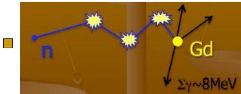
Fast  $n$  recoil on  $p$  (low energy) and captured on  $\text{Gd}$
