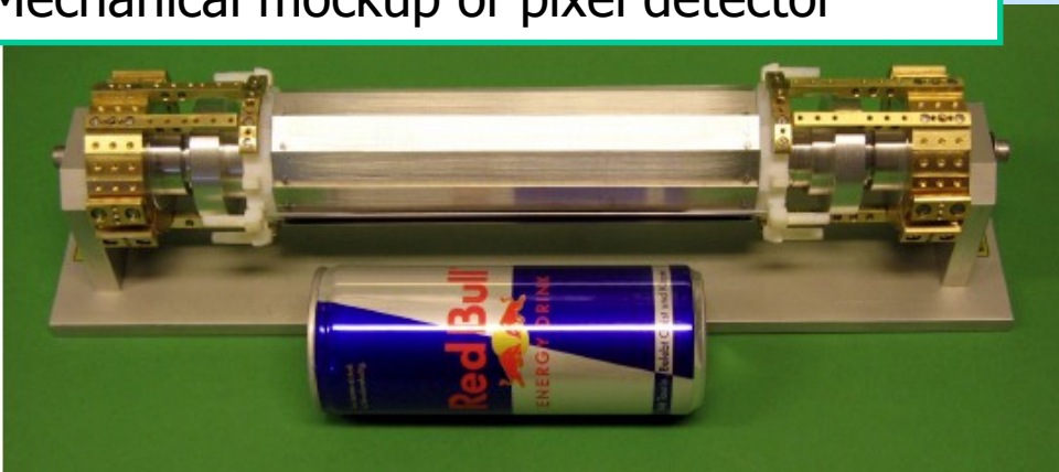
Prototype DEPFET pixel sensor and readout
