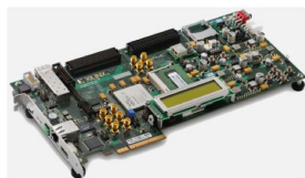
KC-705 low cost board (1700 USD) equipped with the Kintex 7 FPGA
